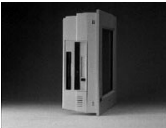
The PPC-140/120's side-mounted FDD, PCMCIA and CD-ROM drives
