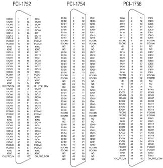
IDO00 ~ IDO15 :Isolated digital output of Group 0 IDO16 ~ IDO31 : Isolated digital output of Group 1 IDO32 ~ IDO47 :Isolated digital output of Group 2 IDO48 ~ IDO63 :Isolated digital output of Group 3 PCOM0 : External common input of Group 0 PCOM1 : External common input of Group 1 PCOM2 : External common input of Group 2 PCOM3: External common input of Group 3
