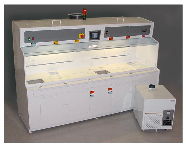
The Manual Etch Bench is constructed of 1/2" FM 4910 approved, white PVC-C, measuring 108"W x 52-1/4"D x 84-7/8"H. Station includes four PVDF process tanks and two quick dump rinse tanks, each measuring 11-1/4"W x 11-1/4"L x 11-3/4"D. Process tanks are recirculated. filtered and temperature controlled with 360° overflow, inlet diffusion sparger, tank leveling capability, liquid level sensor, chemical bulk fill and/or DI fill, and removable covers.
