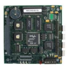
Netsock/310 provides a turnkey,network-oriented platform on which to build embedded systems. Based on the Micro/sys SBC0386EX embedded PC and its built-in Ethernet port, Netsock/310 is a powerful 386EX computer that offers midrange to highrange performance, and that can significantly reduce development time.
