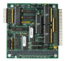
The MPC132 TTL I/O Adapter adds 32 TTL I/O lines to any computer that supports PC/104 I/O modules. The card is organized as four groups of 8 bits each. Each group can be user-configured as an 8-bit input port or an 8-bit output port. In addition, each port can be configured as inverting or non-inverting. Output ports include "readback" capability for simplified bit-oriented control software.
