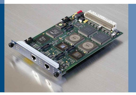
Olicom's CrossFire<sup>™</sup> 8660 Translational Switch Module is a 2-port expansion module for the CrossFire 8600 and 8605 Token-Ring switches, and is designed to allow Token-Ring to Fast Ethernet networks to be quickly and cost-effectively interconnected.
