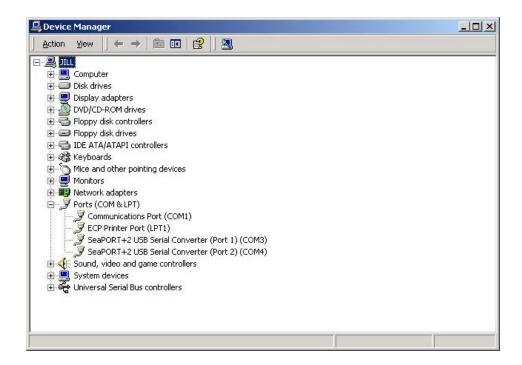
You can access your new COM: ports by using the assigned COM: identifiers as shown above. In this case, it is COM 3 and 4. However, this assignment will vary from system to system. At this point, the hardware is recognized and ready to use.
