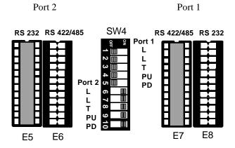
Figure 3: Electrical Interface Configuration
