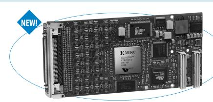
Download your own logic programs and algorithms into the on-board user-configured FPGA to quickly create a custom digital I/O module.
