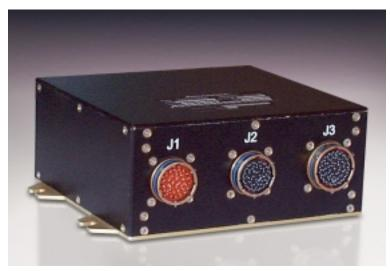
Not just a camera controller, the VCU-05 can accept and switch any standard video source. The VCU-05 contains a 8 x 1 video switcher for direct selection of any video input and also passes all eight channels to interface to cabin video distribution system. The VCU-05 functions can be controlled via basic keyline and/or external RS-485 data bus control. Weighing in at 3.5 lbs. max., the VCU-05 also is able to interface the camera system to a Securaplane® aircraft security system.
