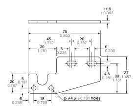
Material: Cold rolled carbon steel (SPCC) (Uni-chrome plated)
