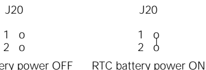
Figure 2.14 RTC standby battery power switch
