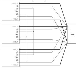
Ensure output power leads are of equal length and type for all units and that they are capable of carrying the load current. Set all units to the required output ±0.1V. The voltage setting pot on unit 1 can be used to set the overall output voltage if required.
