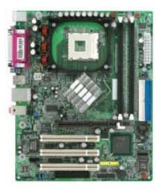
The G4S300-B revision controlled motherboard offers the combination of the Intel® Pentium® 4 or Intel® Celeron® processor power (478 pin), with three PCI slots and 1 AGP 1.5V slot. This MicroATX motherboard has a great combination of on-board audio, on-board video, on-board LAN, and up to 8 USB 2.0 ports.
