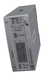
As modular PROFINET IO device the gateway integrates any subordinate SmartWire-DT network into PROFINET. Each SmartWire-DT station is represented as a subsequent slot in the IO device. The cyclic process data is exchanged transparently in between both networks. 1000 bytes of process input/output data can be exchanged with up to 99 SmartWire-DT stations.
