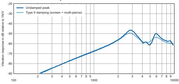
Response measured under constant Voltage drive (at nominal drive) using 10mm x 1mm tubing into 2cc coupler
