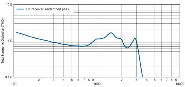
Response measured under constant Voltage drive (0.15mVA at 1kHz) using 10mm x 1mm tubing into 2cc coupler
