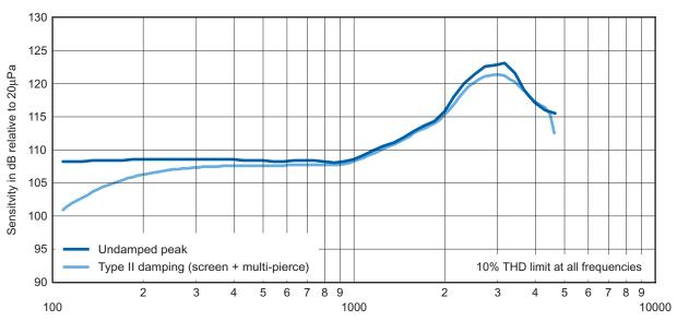
Response measured under constant Voltage drive using 10mm x 1mm tubing into 2cc coupler
