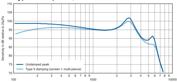
Response measured under constant Voltage drive (0.155mVA at 1kHz) using 10mm x 1mm tubing into 2cc coupler
