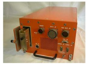
MRC-150 can run MS-DOS, SCO UNIX, QNX, WINDOWS 95 or another operating system designed for the PC.
