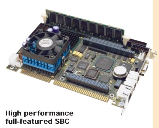
The VIPer830 half-size SBC features a 64-bit Intel Celeron™ processor with on-die 128 KB L2 pipelined burst cache (full CPU core speed, ECC capable). It supports up to 256 MB memory, high performance PCI Ultra DMA/33 IDE and CompactFlash™.
