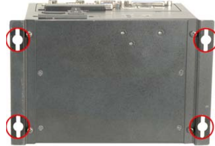
Figure 31: Wall Mounting Holes
