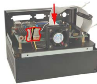
Figure 19: SBC Power Cable and 2.5" HDD Ribbon Cable
