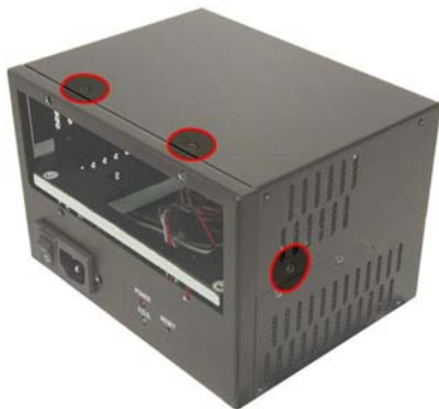
Figure 2: Top Cover Retention Screws on the Top and Sides
