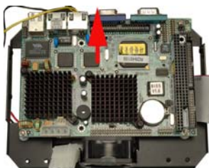
Figure 13: I/O Connectors Direction
