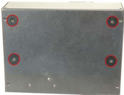
Figure 8: PSU Retention Screws
