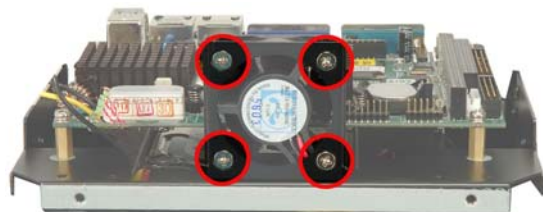
Figure 28: Fan Retention Screws
