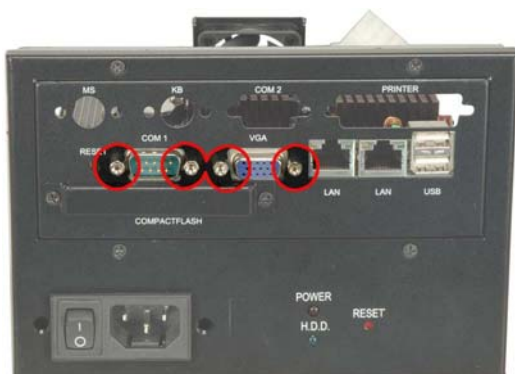
Figure 18: I/O Connector Barrel Screws
