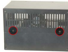
Figure 3: Top Cover Retention Screws at the Rear
