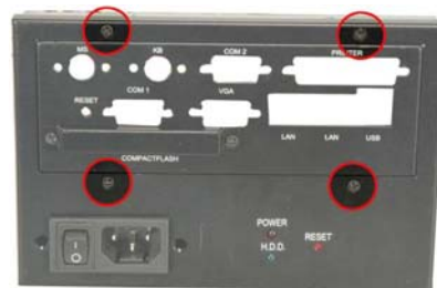
Figure 14: I/O Bracket Retention Screws
