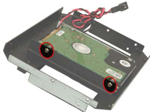
Figure 10: 2.5" HDD Retention Screws
