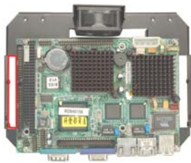
Figure 15: The Hole in the Right Side of the Internal bracket
