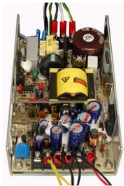
Figure 7: Connect the Power Cables to the Terminal Blocks
