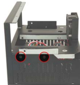
Figure 4: Internal bracket Retention Screws
