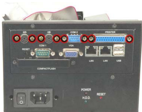
Figure 25: I/O Connector Retention Screws
