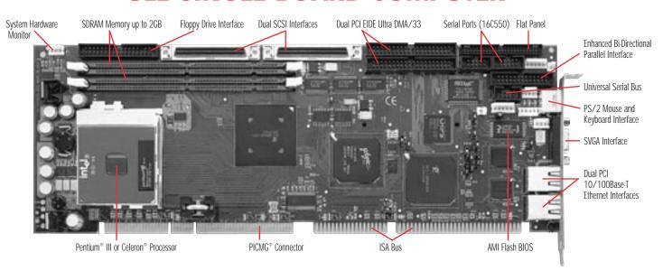
Designed to give you the faster performance and flexibility you need, the ULE has dual Ethernet, dual SCSI, video, SDRAM memory, and an Intel® Pentium® III or Celeron® processor. Additionally, the ULE supports Flat Panel and Compact Flash™. With all of these options on board, the ULE saves you slots and lets you take advantage of the SBC's flexible processor options.
