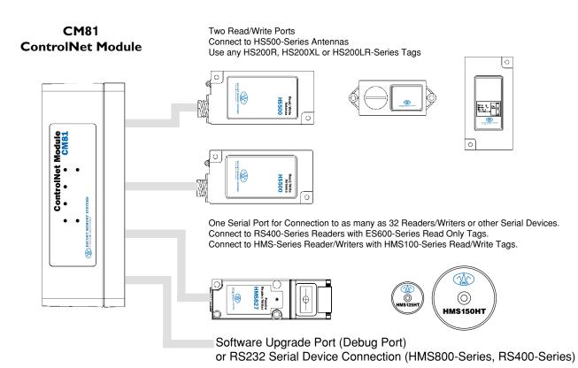
**Available Models** Model Description CM81 ControlNet Communication Module, NEMA 4 (IP66) CM82 ControlNet Communication Module, NEMA 2 (IP31) Accessories Model Description 10-7268 Connector Kit (CMx1) CBL-1439-01 CMx1 to HS500 Cable (1 meter length) CBL-1439-03 CMx1 to HS500 Cable (3 meter length) CBL-1439-06 CMx1 to HS500 Cable (6 meter length) CBL-1439-30 CMx1 to HS500 Cable (30 meter length)
