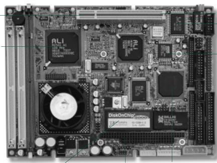
DiskOnChip® 2000 supports TrueFFS® up to 72 MB PC/104 Connector CHIPS® 69000 Flat Panel / CRT SVGA controller
