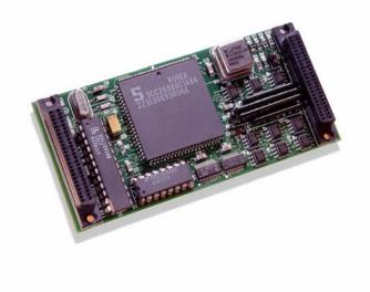
The IP-Octal-485 IndustryPack module implements eight EIA-485 asynchronous serial ports, each with DX+, DX- balanced pair signals and a ground.
