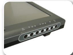
Membrane Keypad for LCD On/Off, Brightness Down/Up, Volume Down/Up, Lock, Ambient Light Sensor On/Off Control
