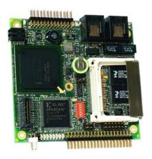
The SBC1626 combines a fast Intel XScale RISC processor, lots of memory, and StackableUSB I/O capability on a small 104™ Form Factor board. The power-efficient ARM architecture means the SBC1626 draws little power at its full 533MHz clock speed, thus reducing the power supply and cooling requirements of the board. On-board I/O includes 24 TTL digital I/O lines, dual 10/100BASE-T Ethernet, CompactFlash, and four (4) serial ports.
