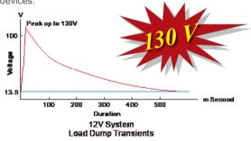
Load dump transients typically reach peak voltages of 130 volts in 12 volt systems with relatively slow rise times.
