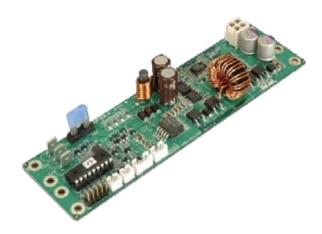
Dedicated single 12V Power for Car PC and Battery Powered Applications Designed to provide power and to control the on/off switch of a motherboard based on the ignition status.
