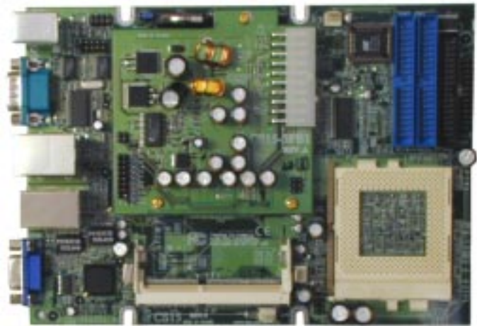
Photograph (GCS15-EN) includes power conversion board which fits above the motherboard. The Illustration shows the location of the power conversion board connector.
