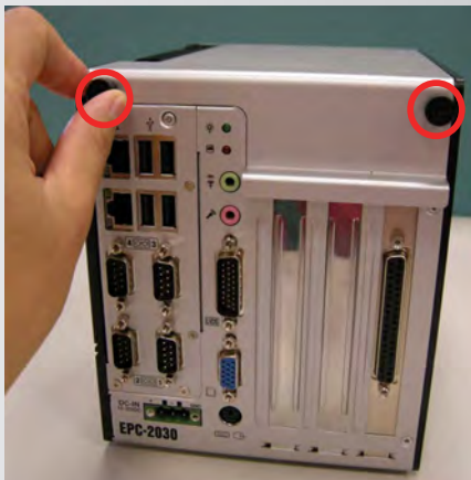
Thumbscrew Design for Easy, Tool-free Installation
