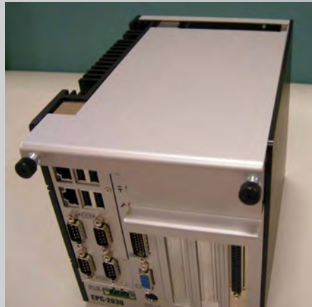
Easily Remove Top Cover by Hand
