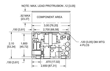
Overall Dimensions: 2.65 x 2.10 x .85 inches 67.31mm x 53.34mm x 21.59mm Weight: 0.25 LBS. [.113 kg]
