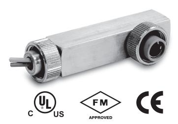
This sensor features a very high temperature sensitivity ultraviolet (UV) tube for monitoring gas or oil flames that cycle on and off frequently. The Eclipse flame safeguard checks for a short-circuited, or "run away" scanner at the beginning and end of each flame cycle.
