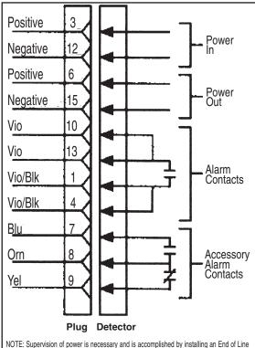
NOTE: Supervision of power is necessary and is accomplished by installing an End of Line Relay Assembly. The EOL Relay Assembly contacts are closed when energized and are wired in series with the alarm loop. Power failure or a break in the power loop de-energizes the EOL Relay, causing the relay contacts to open. This results in a trouble signal at the control panel.
