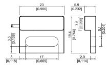
Reed Sensors with Screw Fastening Slot
