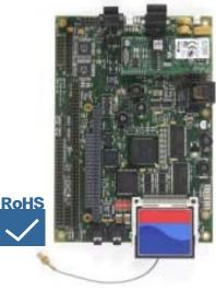
The SBC4670 brings the PXA270 ARM processor to an EPIC form-factor. The efficient XScale board has a maximum 720mA power draw at its full 520MHz speed. This low power draw enables the board to be powered by Power Over Ethernet technology. Other optional serial protocols supported on the SBC4670 include socket modem for GSM/ GPRS or Bluetooth wireless, industry standard CAN, GPS, five serial ports, and 10/100 BASE-T Ethernet. Extended temperature operation is available.
