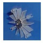
Wakefield's new 882 series heat sinks can be used with LEDs in the star package from Lumileds, Osram, and others. The radial design and fin area is ideally suited for natural convection applications such as ceiling lighting. A fan can also be used for increased performance in a forced convection application. Three sets of mounting holes allow maximum flexibility.
