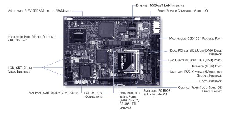
The highly integrated Little Board™ P6d EBX-compatible SBC features a powerful 333 MHz Mobile Pentium II "Dixon" processor, advanced networking, high-performance graphics, SoundBlaster™-compatible sound and ECC memory option. Ideal for ruggedized embedded designs with demanding multimedia performance requirements, it also provides 10/100BaseT Ethernet and 3D graphics for both CRTs and flat panel displays.
