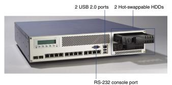
2 PCI-X Removable fans expansion slots Power supply LAN expansion board PCI express PCI expansion
