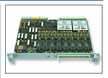
**Built-in-Testing:** Built-in-Test logic provides the user with the capability to test all of the active components on the board, including the output switches. This test scheme utilizes an on-board analog-to-digital converter (ADC) and multiplexers, as shown in Figure 1.
