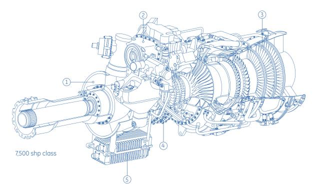
(1) Corrosion-resistant materials throughout the engine to operate in the marine environment (2) Modular engine with sealed oil sumps and accessible gearbox for ease of field maintenance (3) Modern turbine aerodynamics, materials and cooling schemes for durability and efficiency (4) Rugged compressor with split casing and erosion coating to increase repair intervals (5) Engine-mounted FADEC with prognostics and health management to improve performance and reduce maintenance cost
