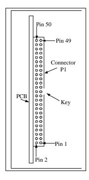
The connector mounted on the board is manufactured by Tyco and has the part number AMP 1-103311-0. The part number of the mating connector is AMP 1-746285.
