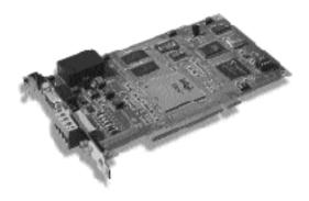
The SST Profibus PCI card connects your PCI bus computer to Profibus DP, FMS client\*, FDL and the S7 Communication Port.
