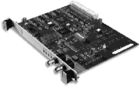
The SST Reliance AutoMax VME card connects your VMEbus computer to a Reliance AutoMax DCS or Remote I/O network.
