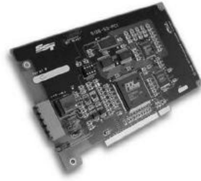
The SST Data Highway Plus PCI interface card connects your PCI bus computer to a Rockwell Automation's Data Highway Plus (DH+) network.
