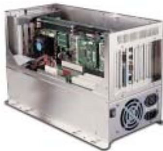
ACS-2307 Control box 7-Slot PICMG backplane with 3 x PCI, 3 x ISA, 1 x PICMG slots
