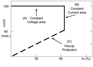
Typical LED power supply I-V curve
