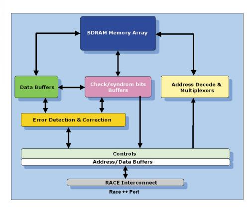
Race ++ SDRAM Controller (used in the MM-6194D & MM-6494D)
