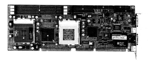
The dual Socket 370 IAC-F372L is a full-size PICMG Single Board Computer (SBC) that supports up to two Intel **Celeron Socket 370** PPGA processors up to 500MHz and higher. This gives you near Pentium II level performance with less heat build up and a lower cost. Built on the **Intel 440BX AGPset**, the IAC-F372L can run at either 66MHz or 100MHz FSB, which means that when Intel creates new faster processors for socket 370, you will be ready.
