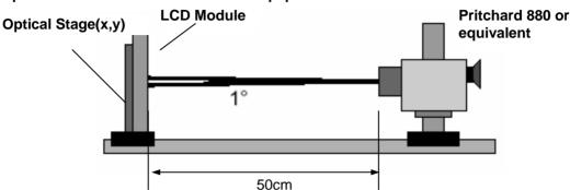
Table 8. OPTICAL CHARACTERISTICS (Ta=25 °C, V<sub>CC</sub>=20.0V, f<sub>V</sub>=60Hz, Dclk=125MHz, I<sub>BL</sub>=7.0mArms)
