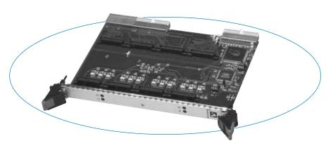
Mix and match plug-in modules with different I/O functions to quickly create custom I/O boards with hundreds of channels.
