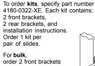
For **bulk**, order 2 front brackets (P/N 4010-0516-CE) and 2 rear brackets (P/N 4080-0508-CE) per pair of slides.
