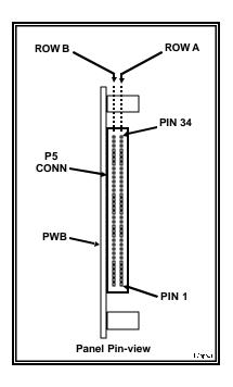
The 68-pin DSUB (user I/O interface) connector (PLUG) is mounted at the front edge of the board (Ref. Des. PA2, for row A & PB2, for row B). The part number is P50E-068PI-SRI-TG, manufacturer, Robinson Nugent. The mating part number is P50E68-S-TG. This cable is used for all 4 channels. The Robinson Nugent phone no. is 812-945-0211. Contact GSC for factory built cables of any desired length. See Table above for pin-out.
