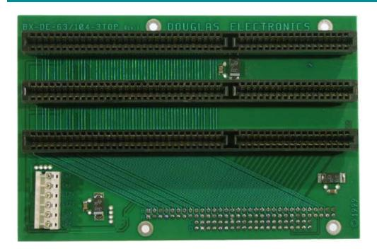
The BX-DE-63/104-3TOP board provides slots for up to three ISA boards on the top of a PC/104 stack
