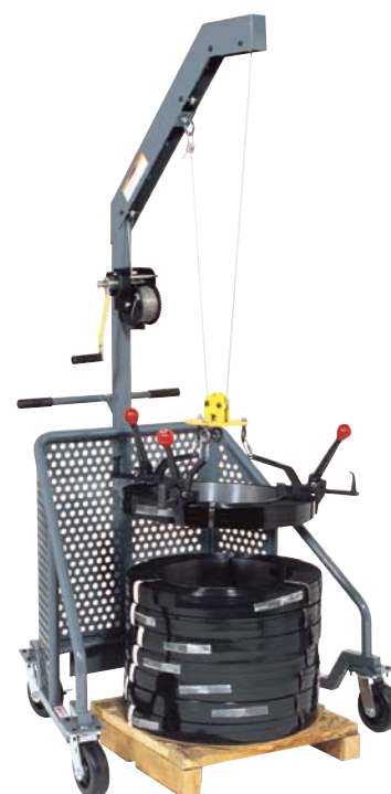
Coil Lifter Capable of lifting up to 125 lb. strap coils, the standard coil lifter is designed for easy dispenser loading, both vertically and horizontally. Accommodates both mill and ribbon wound steel strap coils as well as standard plastic coils. Available in a stationary (Part No. 425650) or portable model (Part No. 424700).
